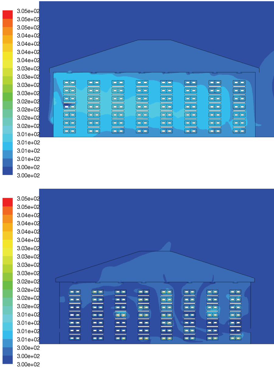
Contours of Static Temperature (k) Mar 18, 2006 FLUENT 6.2 (2d, dp, segregated, spe, rke)
