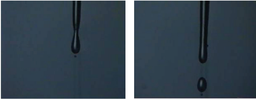
Fig. 3. Bubble pinch-off type of GE phenomena
