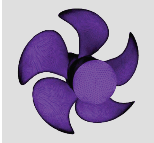
Fig. 3. Marine Propeller 5168 and Surface Mesh
